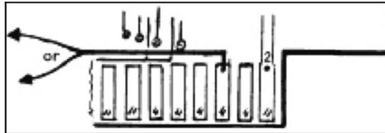
Connect other end of wire to pin 6 of card-edge, i.e., the 3rd lead from the right on the COMPONENT side of the PC board.
